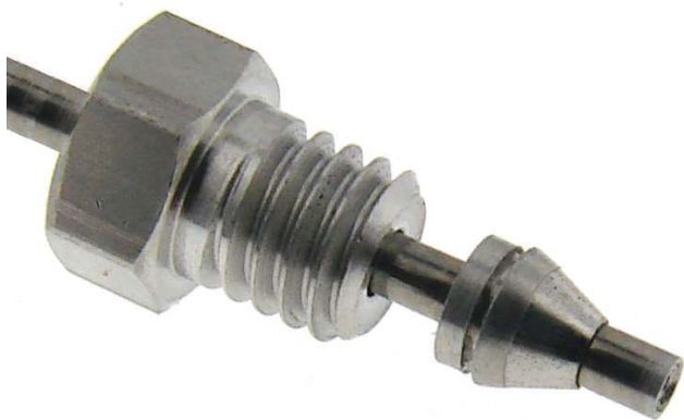
Fig. 6: Pre-swaged ferrules and compression screw. In this case, the ferrules have been over-tightened, as evidenced by the rear ferrule, which is no longer free to rotate, and by the slight discoloration covering the bottom 2/3 of the front ferrule. In a properly tightened assembly, there would only be a small band of discoloration at the tip of the ferrule, indicating the “line contact” compression
