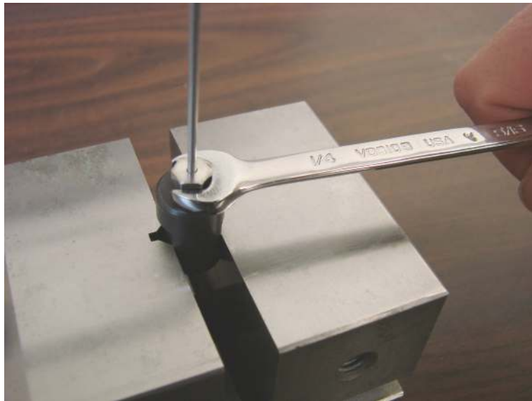
Fig. 5: Compression fitting assembly using a pre-swage tool in a vice
