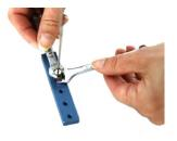
9.) Using a pair of wrenches (one on the nut, and one to support the body of the fitting) tighten the nut an additional 1/8 to 1/4 of a turn, (45 to 90) degrees.
