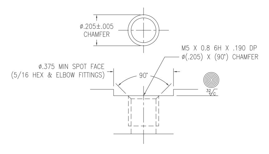
INSTALLATION TORQUE: BRASS FITTINGS - 7 TO 9 IN\*LBF STAINLESS STEEL FITTINGS - 9 TO 12 IN\*LBF
